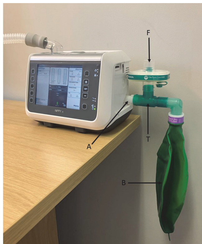
Abstract P110 Figure 1 Breas® Nippy 4+ ventilator with modification fitted. Legend: B = reservoir bag, F= bacterial filter, A= adaptor, T= T-piece connector
