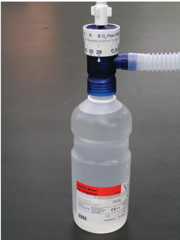
**Figure 18** Large volume nebulisation-based humidifier.
